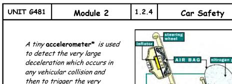
deceleration which occurs in any vehicular collision and then to trigger the very rapid, explosive inflation of the air-bag.
