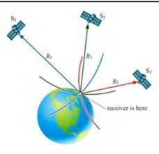
The receiver's position is somewhere on the circle produced by the intersection of the two spheres. It is the distance  $R_3$  from satellite  $S_3$  which pinpoints the receiver's actual location on the circle.
