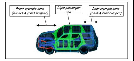
Other parts of the car, such as the **passenger cell**, are designed as a very strong, rigid compartment so as to maximise passenger protection in the event of a collision. Another interesting feature is the design of the engine support brackets which will shear in the event of a crash, directing the heavy engine downwards and so preventing it from penetrating the passenger compartment.
